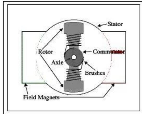
magnetic field. As you are well aware of from playing with magnets as a kid, opposite (North and South) polarities attract, while like polarities (North and North, South and South) repel. The internal configuration of a DC motor is designed to harness the magnetic interaction between a current-carrying conductor and an external magnetic field to generate rotational motion.
