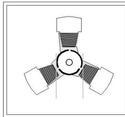
There's probably no better way to see how an average DC motor is put together, than by just opening one up. Unfortunately this is tedious work, as well as requiring the destruction of a perfectly good motor. The guts of a disassembled Mabuchi FF-030-PN motor (the same model that Solarbotics sells) are available for (on 10 lines / cm graph paper). This is a basic 3-pole DC motor, with 2 brushes and three commutator contacts.
